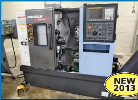
Doosan Model Lynx 220A Slant Bed CNC Turning Center
