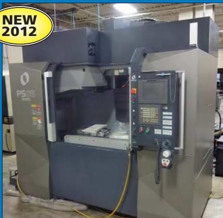
Makino Model PS95 High-Speed Heavy-Duty CNC VMC
