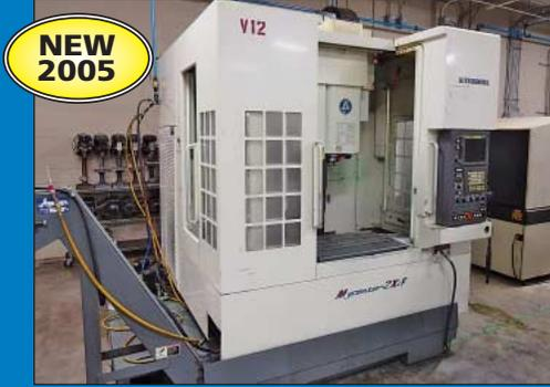
Kitamura Mycenter 2Xif CNC Vertical Machining Center
