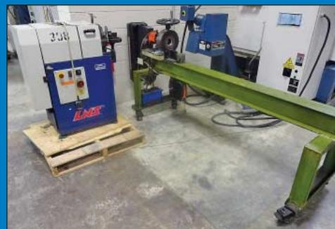
3" LNS Model PB-80 Chamfering Machine & 3" Custom Bar Chamfering Machine with 8" Chuck, 6" Rail Support
