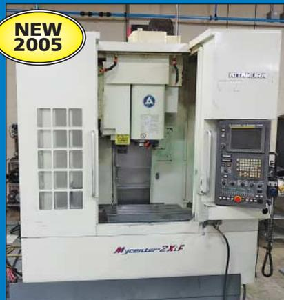
Kitamura Mycenter 2Xif CNC Vertical Machining Center
